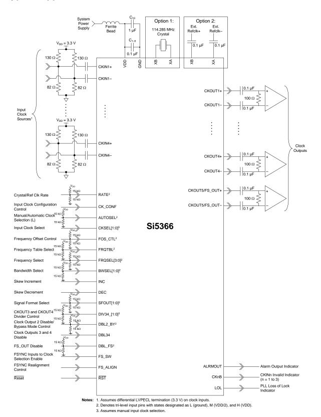
Figure 4. Si5366 Typical Application Circuit
