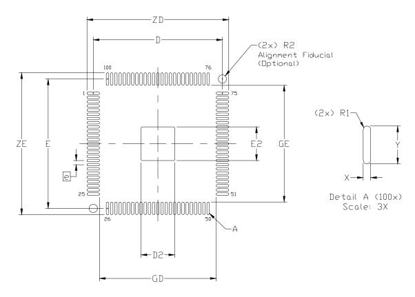
Figure 6. PCB Land Pattern Diagram
