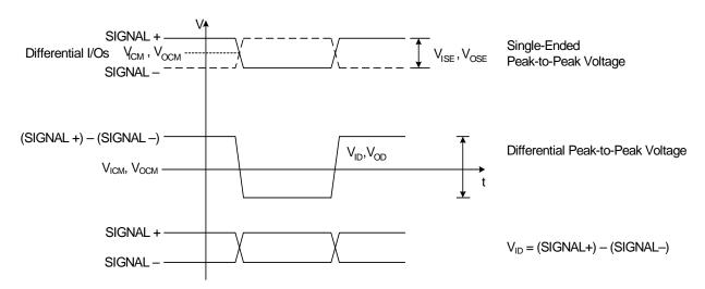
Figure 1. Differential Voltage Characteristics
