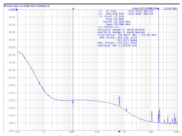
Figure 3. Typical Phase Noise Plot
