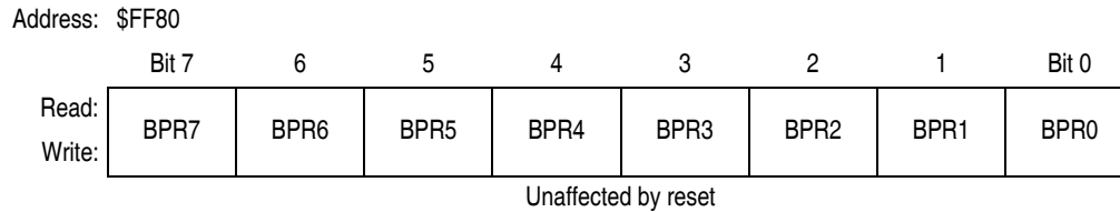
Figure 2-4. FLASH-1 Block Protect Register (FL1BPR)
