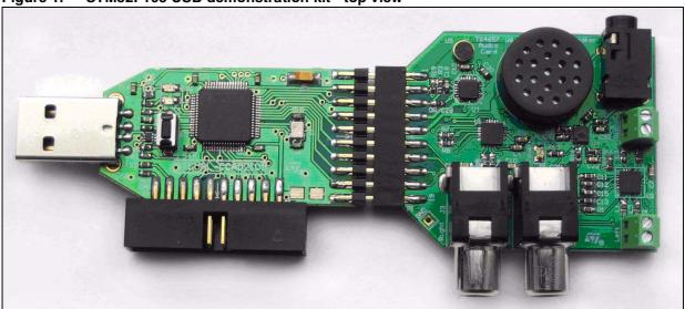
Figure 1. STM32F103 USB demonstration kit - top view
