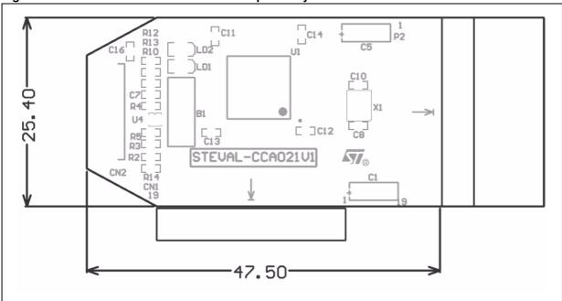
Figure 27. STM32F103 controller board - bottom overlay
