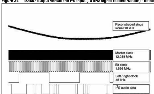
Figure 24. TS4657 output versus the I<sup>2</sup>S input (10 kHz signal reconstruction) - detail
