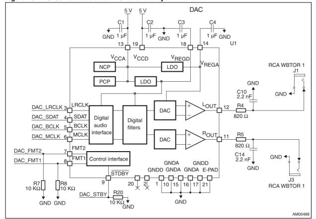
Figure 19. TS4657 stereo audio DAC functionality
