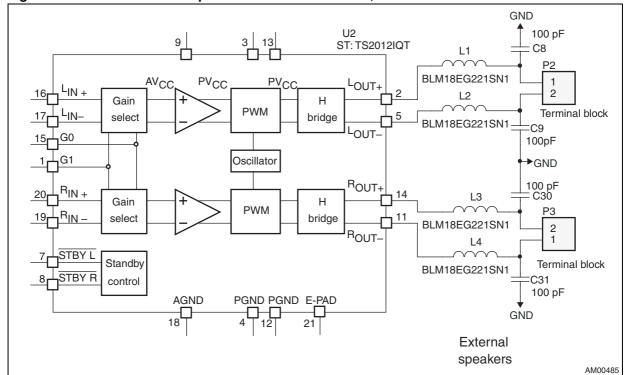
Figure 16. TS2012 stereo output terminal connectors P2, P3
