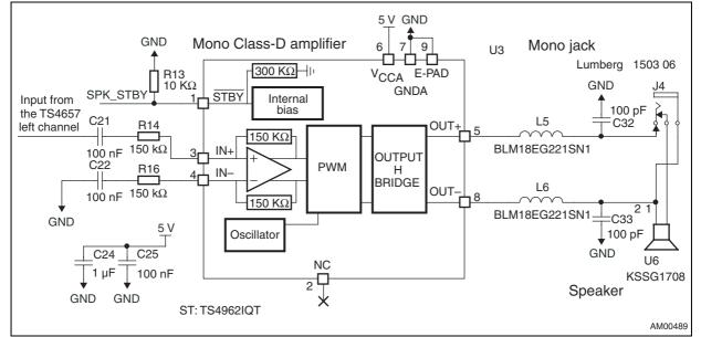
Figure 20. TS4962 mono Class-D amplifier functionality
