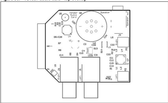
Figure 31. TS4657 audio card - bottom overlay
