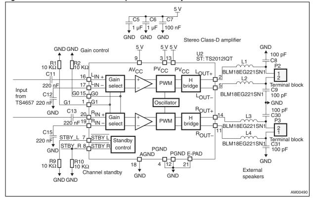
Figure 21. TS2012 stereo Class-D amplifier functionality
