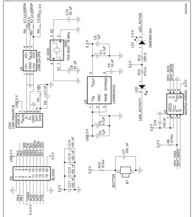
Figure 35. STM32F103 controller board - schematic - part 2
