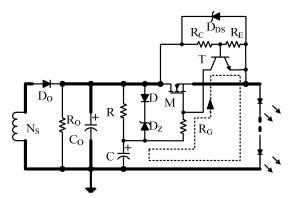
Figure 16: Drain-Source OVP and OCP Circuit
