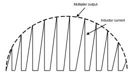
**Figure 4: Power-Factor Correction**
