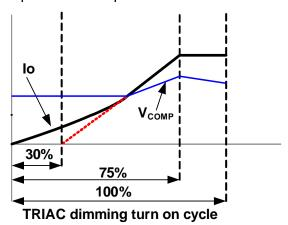
Figure 12: Dimming Curve Analog Dimming
