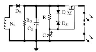
Figure14: Ripple Suppressor
