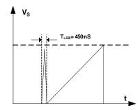
Figure 7: Leading-Edge Blanking
