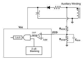
Figure 8: OVP Sampling Circuit
