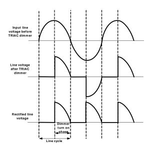
Figure 10: TRIAC Dimmer Waveforms
