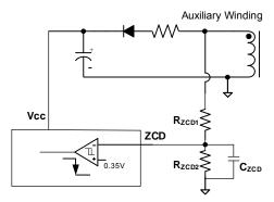
**Figure 3: Zero-Current Detector**
