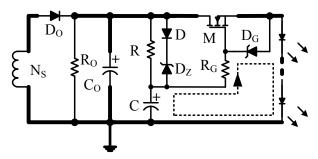
Figure 15: Gate-Source OVP Circuit
