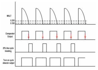
Figure 11: Dimming Turn-On Cycle Detector
