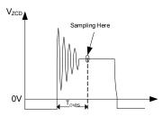
Figure 9: ZCD Voltage and OVP Sampling
