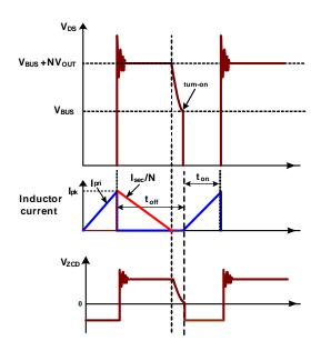
Figure 2: Boundary-Conduction Mode
