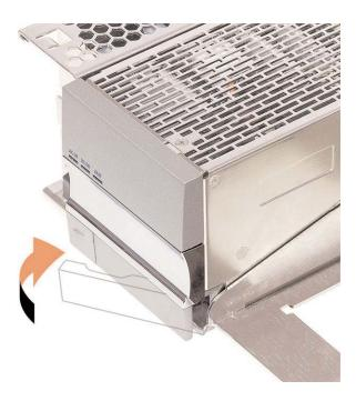
Figure 14 - Power module insertion
