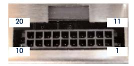
Figure 12 - Alarm and signal connector
