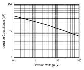
Fig. 5 - Typical Junction Capacitance
