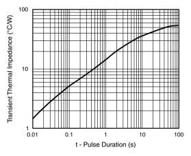
Fig. 6 - Typical Transient Thermal Impedance
