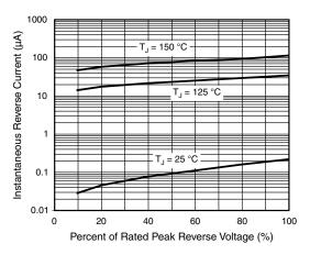
Fig. 4 - Typical Reverse Characteristics
