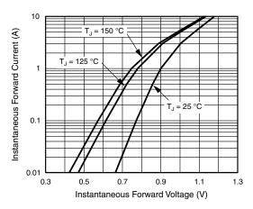
Fig. 3 - Typical Instantaneous Forward Characteristics
