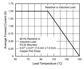
Fig. 1 - Forward Current Derating Curve
