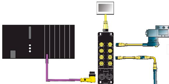
Contained in a 60mm wide housing rated for IP67 environments, BradControl I/O modules can be machine mounted and are able to withstand areas where liquids, dust or vibration may be present. This makes them ideally suited for many applications including material handling equipment and automated assembly machinery.
